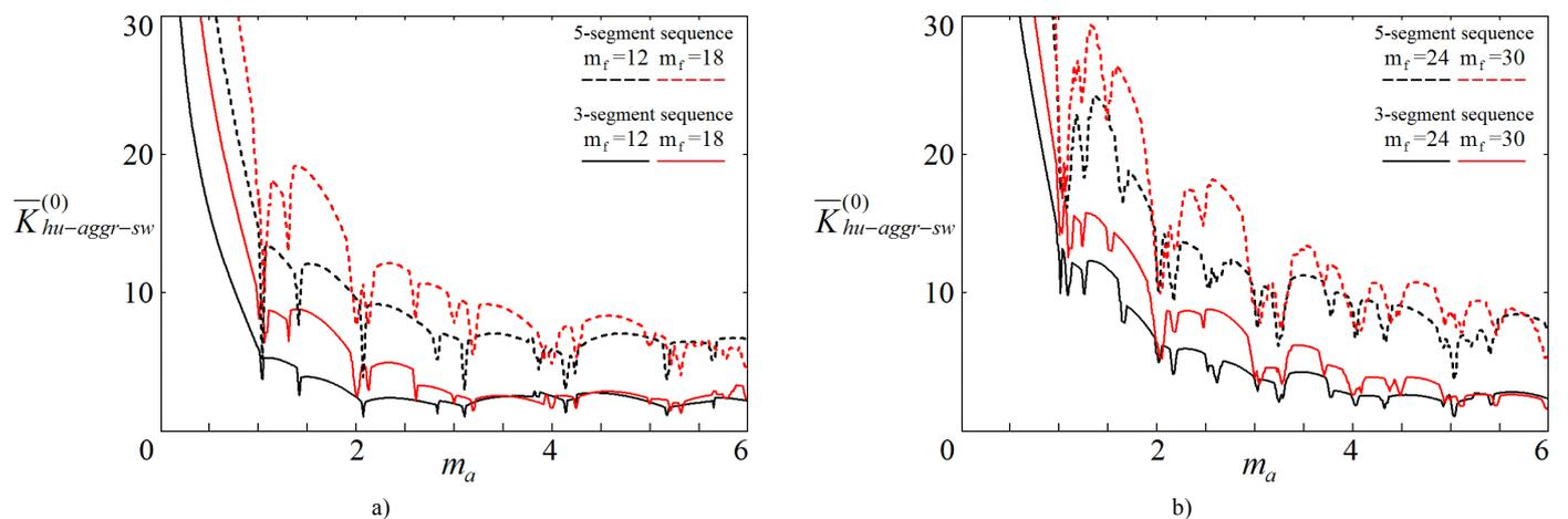
Fig. 7. The zero order aggregate switchings and integrated voltage harmonics factor Mathcad simulation results for the five-segment and the three-segment switching sequences: a) under  $m_f = 12$  and  $m_f = 18$ ; b) under  $m_f = 24$  and  $m_f = 30$ .
