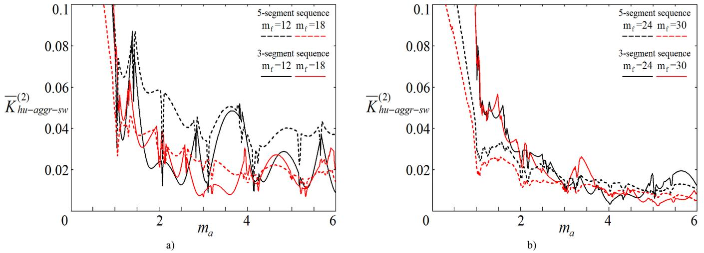
Fig. 9. The second order aggregate switchings and integrated voltage harmonics factor Mathcad simulation results for the five-segment and the three-segment switching sequences: a) under  $m_f = 12$  and  $m_j = 18$ ; b) under  $m_f = 24$  and  $m_j = 30$ .
