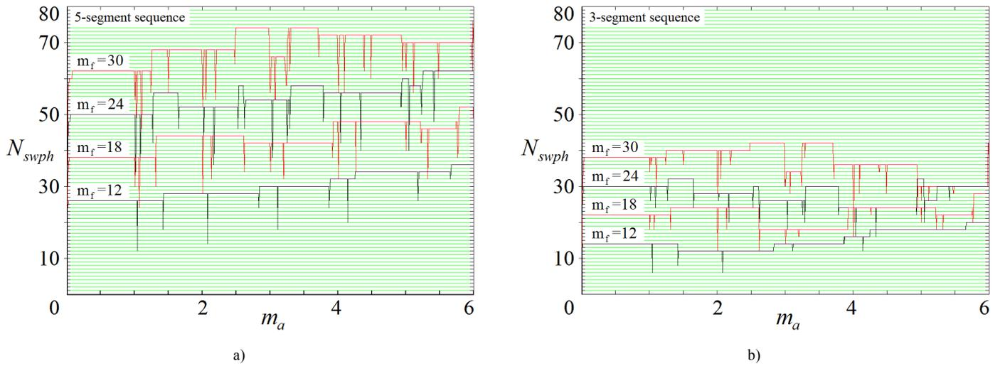
Fig. 4. The Mathcad simulation results of the inverter phase leg switchings numbers: a) for the five-segment switching sequence; b) for the three-segment switching sequence.
