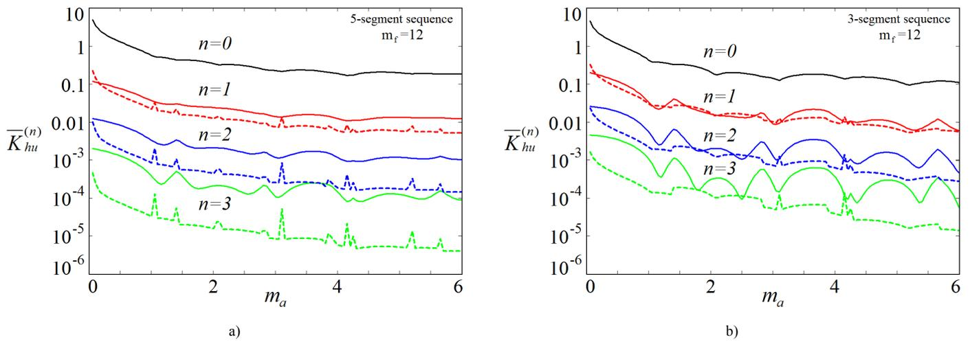
Fig. 5. The Mathcad simulation results of the zero to third orders voltage integral harmonics factors under  $m_f = 12$  a) for the five-segment switching sequence; b) for the three-segment switching sequence.
