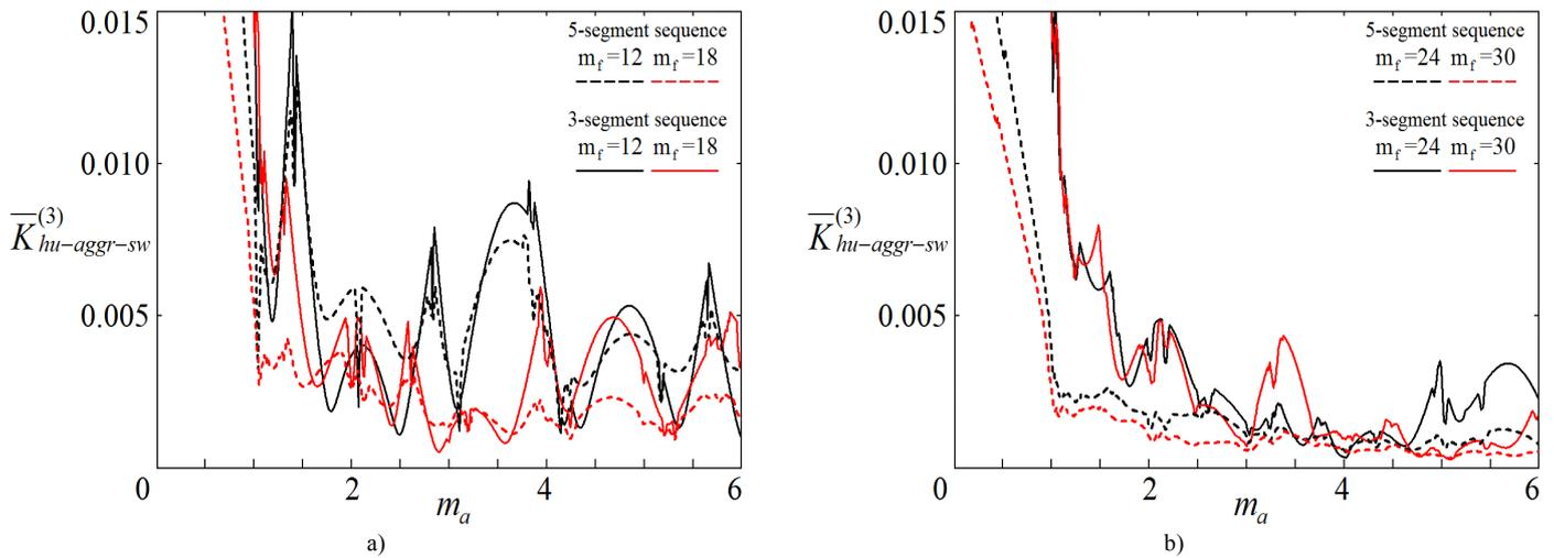
Fig. 10. The third order aggregate switchings and integrated voltage harmonics factor Mathcad simulation results for the five-segment and the three-segment switching sequences: a) under  $m_f = 12$  and  $m_j = 18$ ; b) under  $m_f = 24$  and  $m_j = 30$ .
