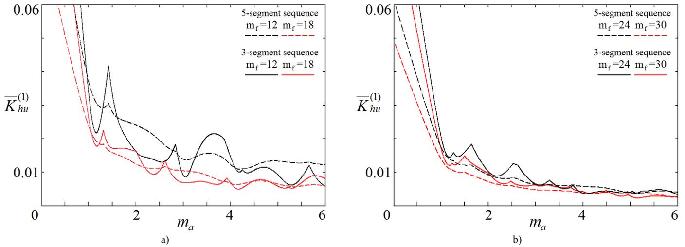
Fig. 1. The first order integral voltage harmonics factor Mathcad simulation results for the five-segment and the three-segment switching sequences: a) under  $m_f = 12$  and  $m_r = 18$ ; b) under  $m_f = 24$  and  $m_r = 30$ .
