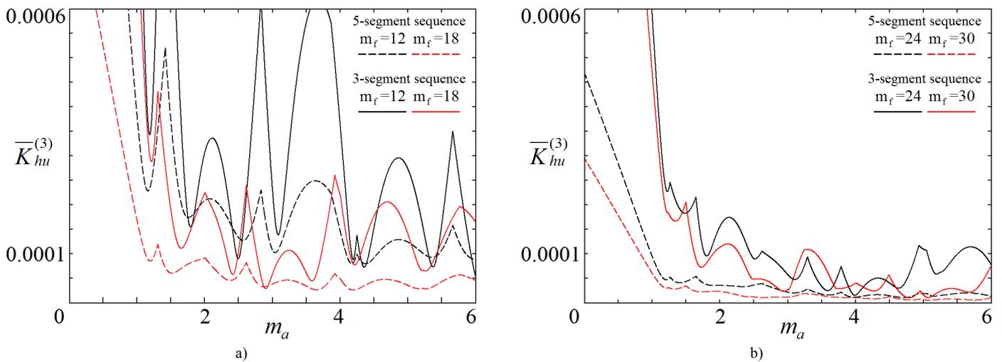
Fig. 3. The third order voltage integral harmonics factor Mathcad simulation results for the five-segment and the three-segment switching sequences: a) under  $m_f = 12$  and  $m_r = 18$ ; b) under  $m_f = 24$  and  $m_r = 30$ .
