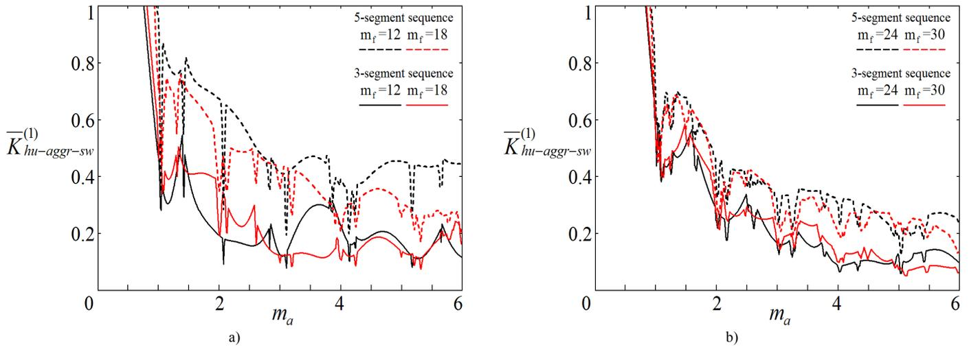
Fig. 8. The first order aggregate switchings and integrated voltage harmonics factor Mathcad simulation results for the five-segment and the three-segment switching sequences: a) under  $m_f = 12$  and  $m_j = 18$ ; b) under  $m_f = 24$  and  $m_j = 30$ .
