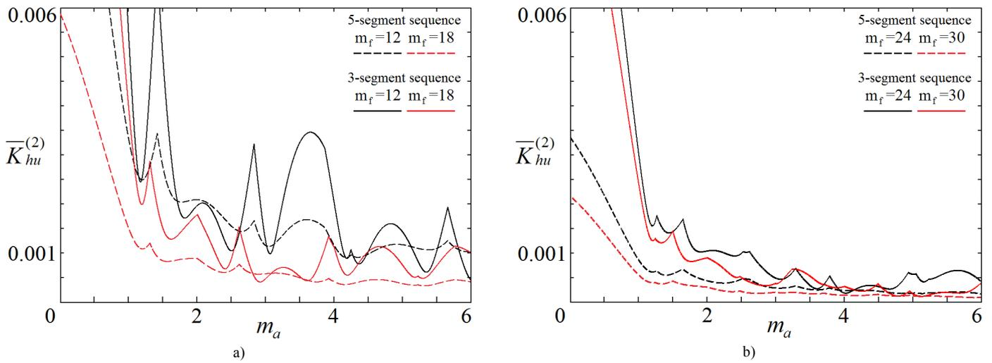
Fig. 2. The second order integral voltage harmonics factor Mathcad simulation results for the five-segment and the three-segment switching sequences: a) under  $m_f = 12$  and  $m_r = 18$ ; b) under  $m_f = 24$  and  $m_r = 30$ .
