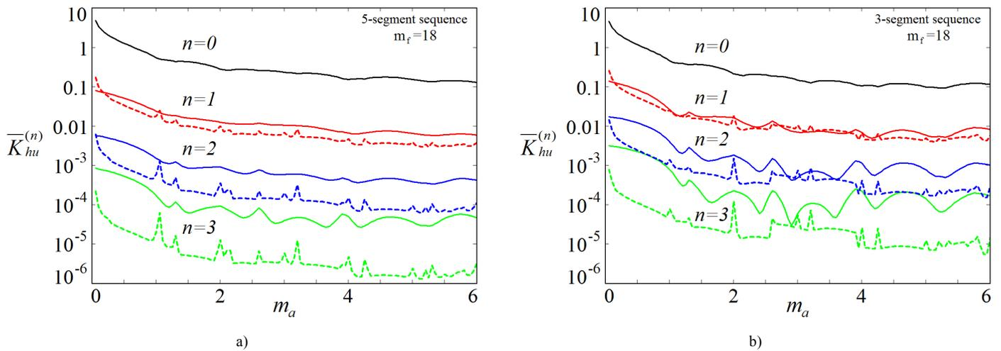
Fig. 6. The Mathcad simulation results of the zero to third orders voltage integral harmonics factors under  $m_f = 18$  a) for the five-segment switching sequence; b) for the three-segment switching sequence.
