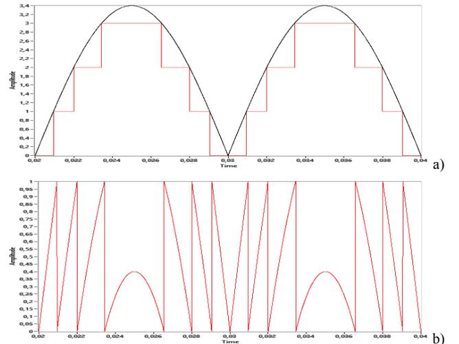
Fig. 2. LabVIEW-simulated POD reference signal for  $m_a = 3.4$ : a) the absolute value (black curve) and its integer part (red curve); b) the fractional part of the absolute value.
