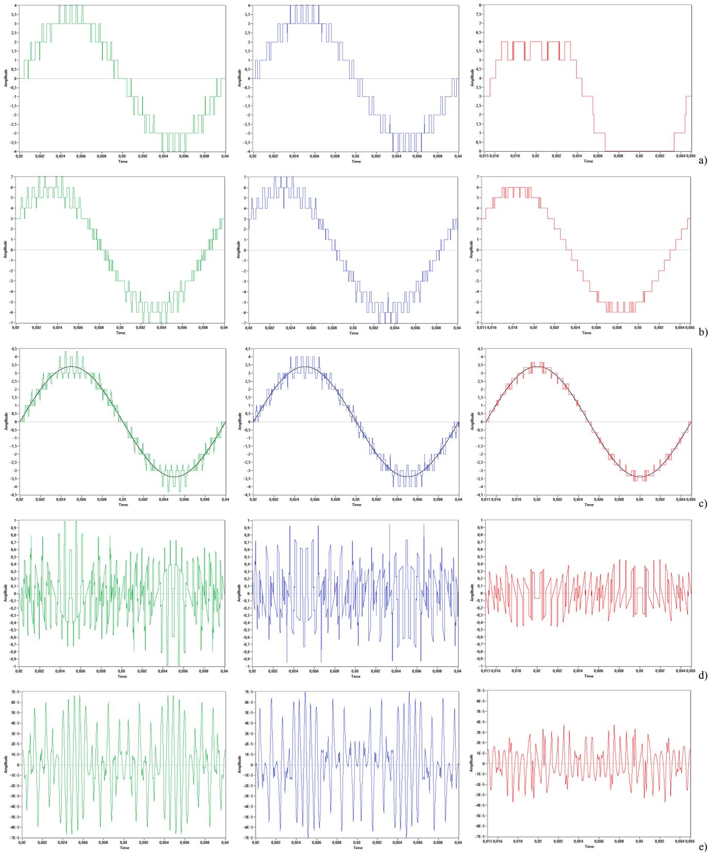
Fig. 3. LabVIEW-simulated output voltages idealized waveforms for the POD-0 (green curves), the POD-180 (blue curves) and the offered SVPWM technique (red curves) under  $m_f = 36$ ,  $m_a = 3.4$ : a) the phase-to-ground voltages; b) the delta voltages; c) the phase-to-neutral voltages and their fundamental components; d) the high harmonics components of the phase-to-neutral voltages; e) the integrated high harmonics components of the phase-to-neutral voltages.
