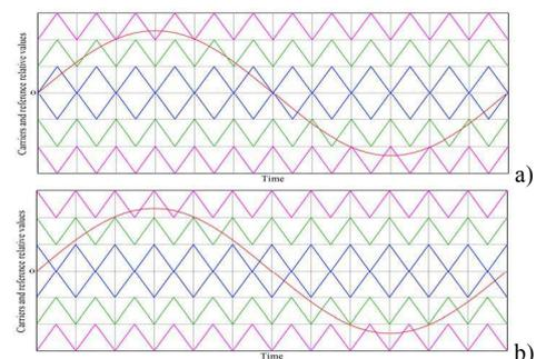
Fig. 1. Carriers and reference waveforms of the phase opposition disposition method: a) POD-0 with 0 degrees phase delay of the positive carriers; b) POD-180 with 180 degrees phase delay of the positive carriers.
