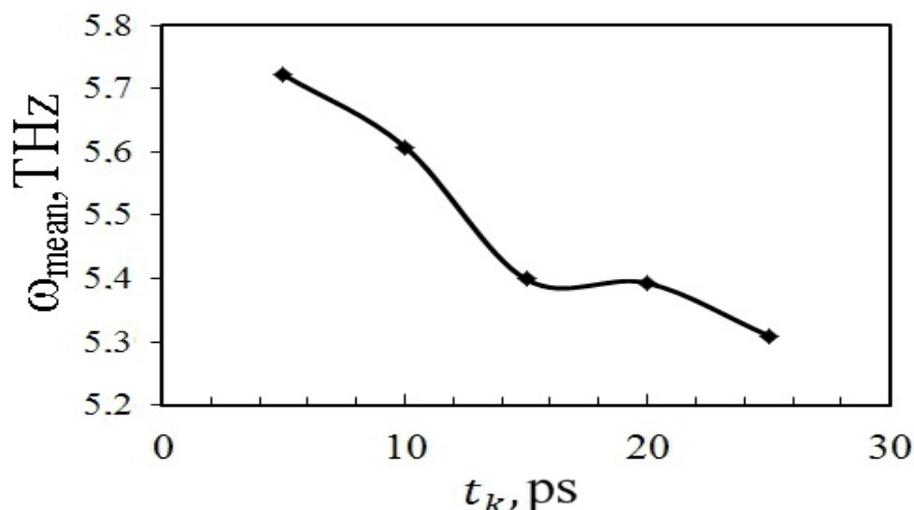
**Fig. 4.** Dependence of the model quasi-breather mean frequency  $\omega_{\text{mean}}$  (in THz) on its lifetime  $t_k$  (in ps)
